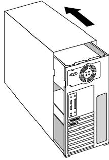
5. If necessary, remove the back panel covers from the slots into which you are installing your Wildcat II 5110 Graphics Accelerator Card, using a Phillips-head screwdriver.
